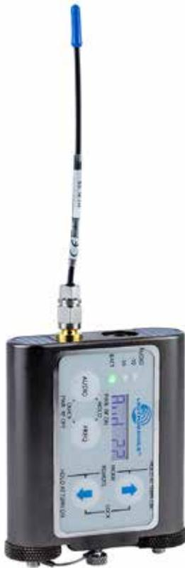
Designed for wet or dusty environments, the WM transmitter features O-ring sealed battery compartments and input jack, a compression sealed antenna port, and gasket sealed control panel and back cover. Dual AA batteries provide twice the operating time of earlier watertight transmitter designs. Larger membrane switches and control panel and a highly visible, backlit LCD enhance the user interface.
