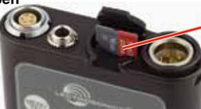
Insert the card with the label facing the keypad side of the recorder.
