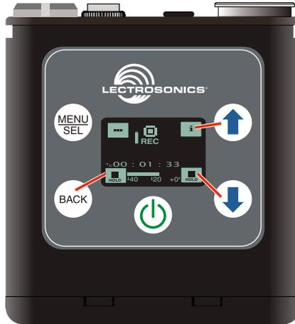
In the Playback Windows, the icons on the LCD change to provide the functions needed during playback. There are three variants of the playback window:
