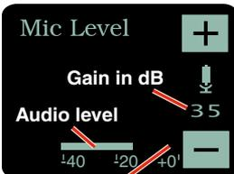
Use the UP and DOWN arrow buttons to adjust the input gain. When the audio level meter reading exceeds the zero at the top, either a “C” or an “L” icon will appear, indicating respectively clipping in the non-safety track (Split Gain mode) or limiting (HD Mono mode). In HD Mono mode, the limiter compresses 30 dB of input level into the top 5 dB, reserved for “overhead” in this mode. In Split Gain mode, the limiter would rarely be engaged, but it will engage if necessary (with no graphical
