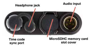
The audio input circuitry is the essentially the same as on Lectrosonics SM and L Series transmitters. Any microphone wired as Lectrosonics "compatible" or "servo bias" will work with the MTCR. (See manual for details.)
