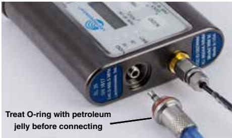
The threaded WP watertight plug on the microphone cable fits into a recessed jack on the top panel. The recess in the opening retains the O-ring when the plug is tightened.
