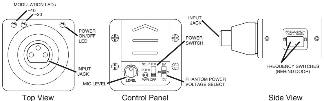
This transmitter may be used with a wide variety of microphones. The 3-pin XLR connector allows the transmitter to be used with any dynamic microphone, as well as many two wire positive bias lavalier systems (such as those systems supplied by Lectrosonics).
