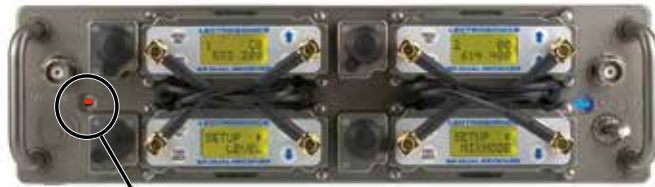
Antenna power switch glows red when DC power is enabled.
