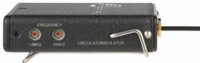
Two 16-position rotary switches adjust the operating frequency over a 25.6 MHz bandwidth in 100 kHz increments. The left switch makes 1.6 MHz steps and the right switch makes 100 kHz steps. A removable stainless steel wire belt clip is provided.
