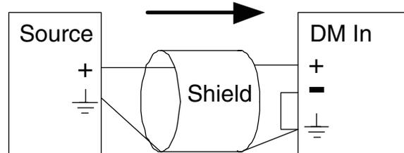
Unbalanced source to DM input
