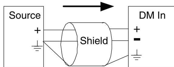
Unbalanced source to DM input
