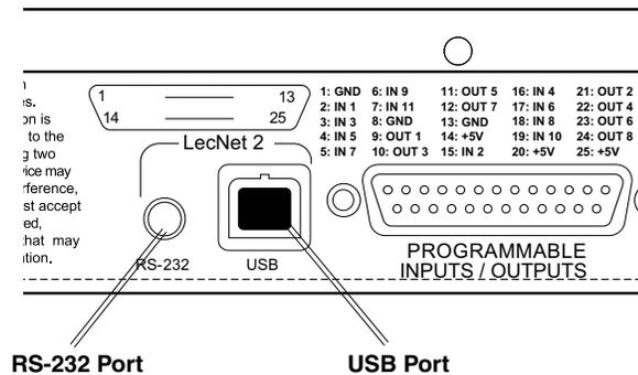
Two RS-232 serial cables are provided. The cable with the **BLACK** TRS connector is an RS-232 cable wired for use with a laptop computer system.
