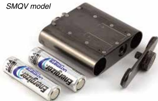
The battery door rotates to open and close on the transmitters. A knurled knob is tightened to maintain pressure on the battery contacts. O-rings around the battery contacts block moisture and dust from entering the battery compartments.
