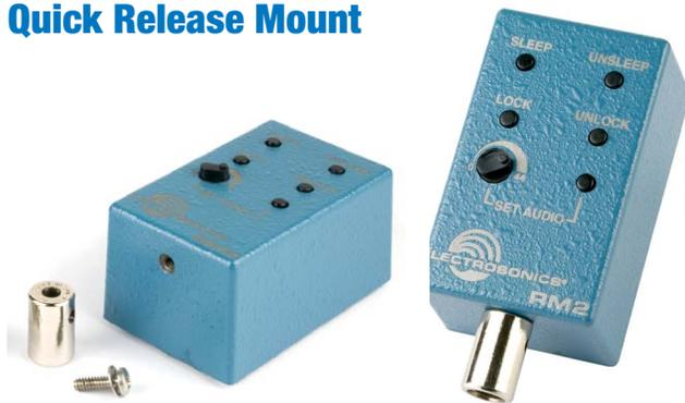
The Phillips head mounting screw fits **inside** the sleeve so that the threads are exposed through the small hole in the sleeve. The screw fits into a threaded insert (PEM nut) in the side of the housing.
