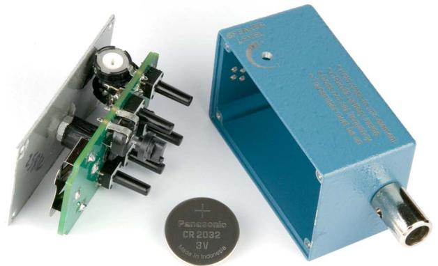
Remove the battery by gripping its edge and pulling it out of the clip. You can also push the battery out of the clip with a toothpick or small tool, but be careful not to damage any of the components mounted on the circuit board.
