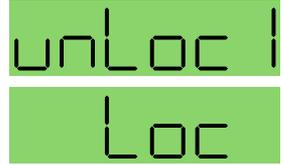
**Important:** The only ways to unlock a locked transmitter are to remove the battery or unlock it via remote. It cannot be unlocked or powered off using the buttons. The remote function will work only if the transmitter was previously configured to respond to remote. The unit will always power up in "unlocked" mode.
