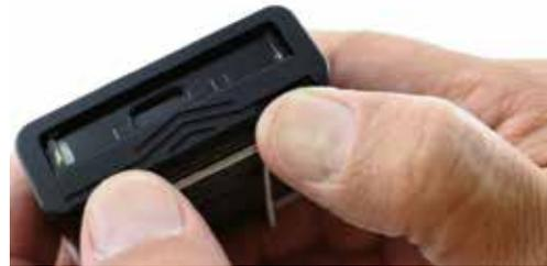
Slide the battery compartment door open, drop the battery in so that the connectors match and slide the battery door closed.
