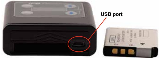
An attached latching door makes battery installation easy. The USB port is located in the battery compartment.
