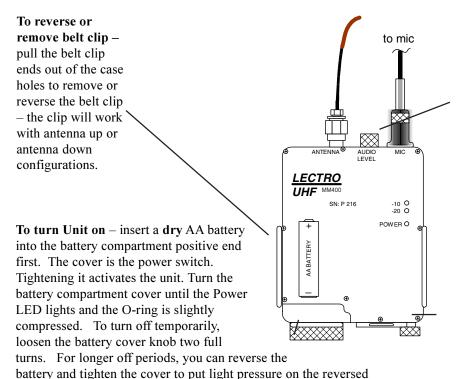
To set the mic level – turn the level adjustment knob (between the antenna and the microphone connector until normal sound levels cause both LEDs to flash green. The LED's turning Red indicates limiting (occasional red is fine).
