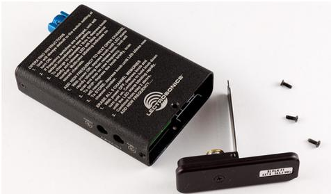
**Step 2:** Remove the central screw at the battery door rotational axis. This will require holding the opposing brass spring-keeper nut with your fingers or pliers to overcome the holding torque of the thread lock adhesive present there.
