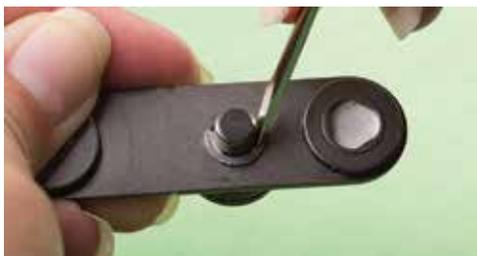
4. Put the new washer onto the new thumb screw and then place them on the door.
