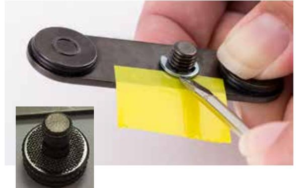
5. Add tape to the door to prevent scratching when applying the e-clip. Install the e-clip onto the thumb screw using a screwdriver. Remove the tape after installing the e-clip.
