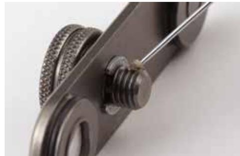
Open the vial and transfer a pinhead speck of silver conductive paste to the second thread from the end of the thumb screw. An easy way to pick up a speck of paste is to partially unfold a paper clip and use the end of the wire to acquire a tiny bit of paste. A toothpick will also work. An amount that covers the end of the wire is sufficient.
