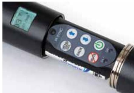
Pressing the power button without holding it for three seconds turns on the transmitter with its RF muted. Similarly, the power button must be depressed for three full seconds to turn it off. The backlit LCD multifunction display on the exterior can be programmed to turn off after 30 seconds, five minutes or to remain lit.
