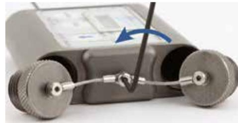
Install new battery caps and tighten the thumb screw **by hand** since it is often removed to recondition (dry out) the desiccant beads.
