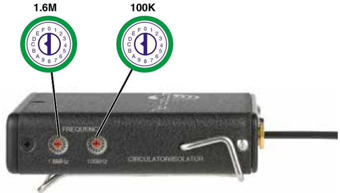
The left switch adjusts the operating frequency of the transmitter up or down in 1.6 MHz steps. The right switch adjusts the operating frequency of the transmitter up or down in 100 kHz steps. It is suggested to use the metering on the associated receiver to find a clear channel. Turn the transmitter off and leave the receiver turned on.
