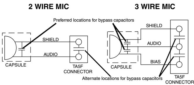
Install the capacitors as follows: Use 330 pF capacitors. Capacitors are available from Lectrosonics. Please specify the part number for the desired lead style.
