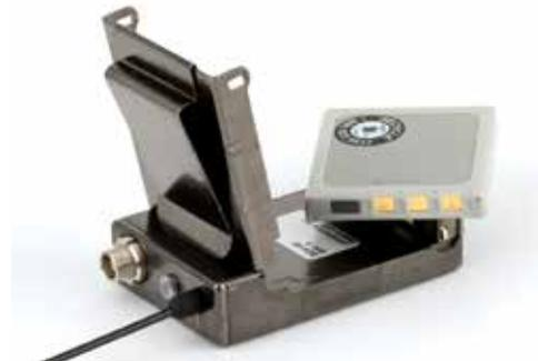
Power is provided by a rechargeable Li-ion battery pack. Spring contacts inside the compartment keep the batteries from rattling and provide reliable electrical contacts. The stainless steel battery door latches securely and cannot be jarred open accidentally.
