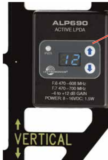
Settings are made with a keypad interface on the control panel.
