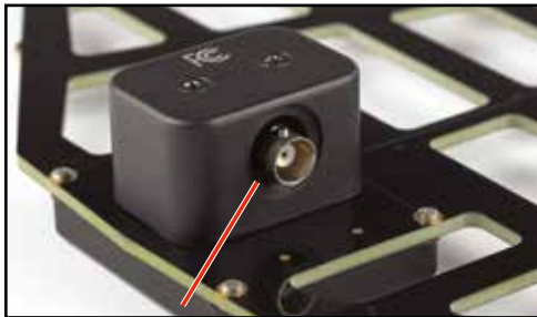
Power is provided by DC bias on the output connector
