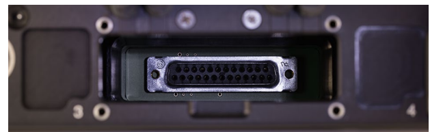
Receivers interface with the Octopack board via a 25-pin connector and the Unislot adapter.
