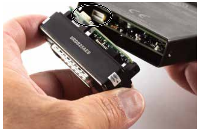
Power and audio connections are made through mating connectors on the adapter and receiver main circuit boards.
