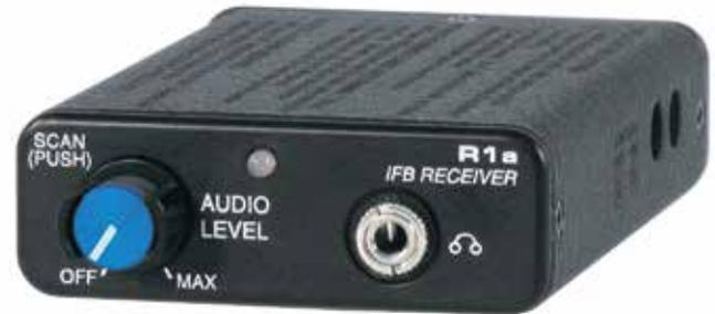
The design uses +/-20 kHz FM deviation for efficient use of the bandwidth, with compandor noise reduction circuitry to increase the signal to noise ratio. A supersonic pilot tone signal controls the audio output squelch to keep the receiver silent when no transmitter signal is received.
