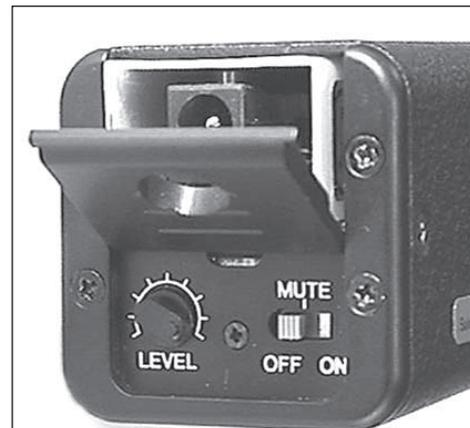
*The HBATELIM kit includes a modified battery door that fits any Lectrosonics “H” type plug-on transmitters.*
