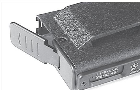
*The MBATELIM model is a kit including the battery eliminator and a modified battery door that fits any Lectrosonics aluminum belt-pack transmitter with a flip-open type door as shown here.*
