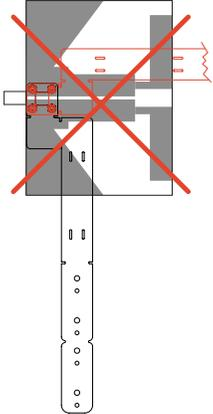
The strap should NOT be mounted so that the long arm is in front of the reflector.
