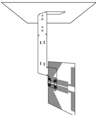
The antenna can also be mounted to a ceiling with appropriate bends in the bracket.
