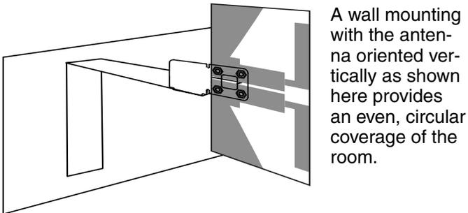
A wall mounting with the antenna oriented vertically as shown here provides an even, circular coverage of the room.
