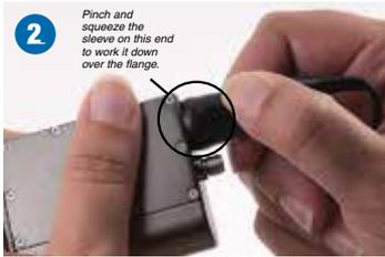
Pinch and squeeze the sleeve near the flange and work it down with a kneading motion over the flange all the way around until it stays in place flush with the housing. Pull on the connector to make sure it is firmly latched.
