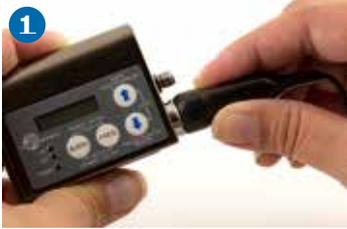
If the sleeve is pulled down and covering the connector, squeeze the end of the sleeve so you can feel the connector inside and press it into the jack until it latches.
