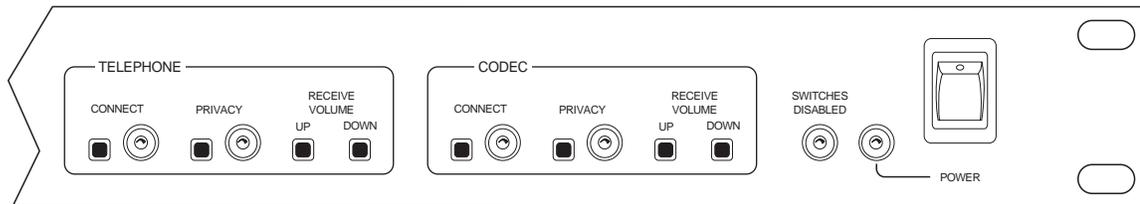
The **CONNECT button** initiates or terminates a connection. The **CONNECT led** indicates an active connection. The telephone connect led flashes when the telephone line is ringing.
