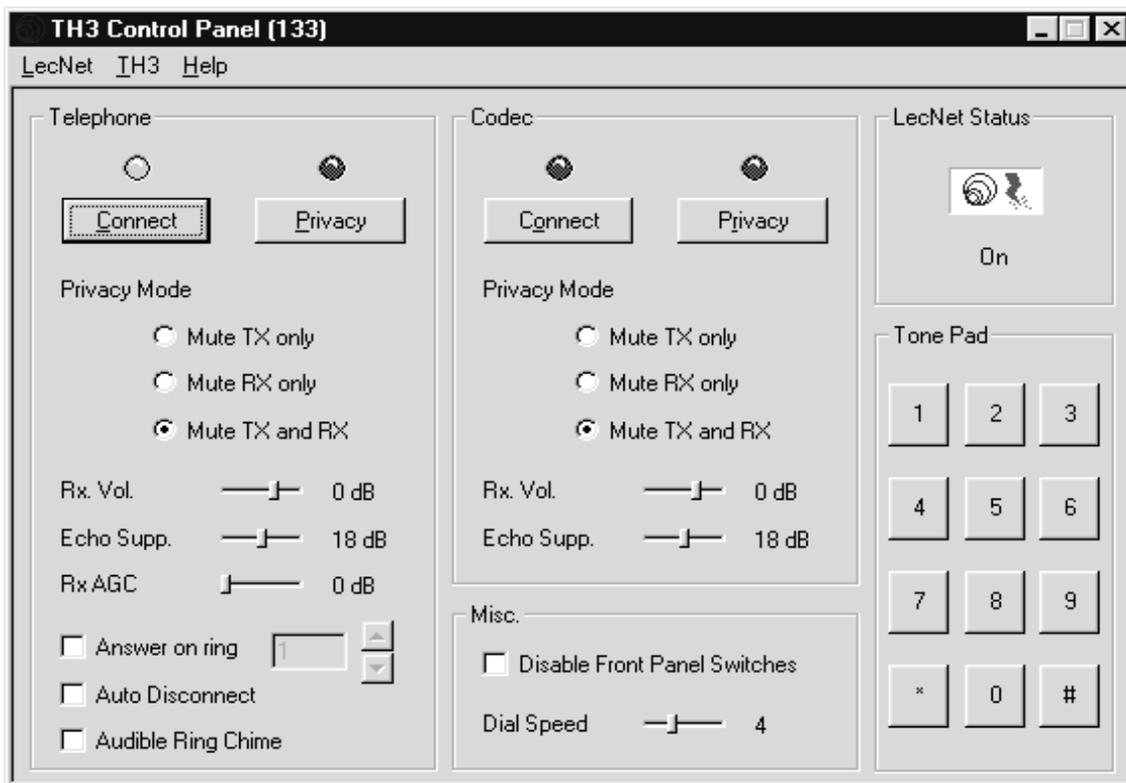
The title bar of the main window includes the word "Demonstration" when the software control panel was invoked directly, as a demonstration of the TH3's features and control panel operation. When the software control panel is or has been actively connected to a TH3, as when invoked via LecNet Master Pro, the TH3's LecNet device address appears in the title bar. This is especially useful if more than one TH3 is being configured simultaneously.
