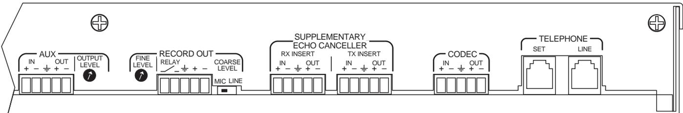
The **AUX interface** provides line level, balanced or unbalanced main input and output from the TH3. Any signal imposed at AUX IN is transmitted to all connected interfaces, and any signal received from connected interfaces is available at AUX OUT, with as little of the transmitted signal as possible. The **OUTPUT LEVEL control** may be used to match the TH3's AUX OUT signal with the level requirements of any attached equipment.
