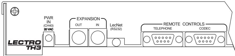
The **PWR IN** jack must be attached to an appropriate power source, such as the included CH40 wall transformer.
