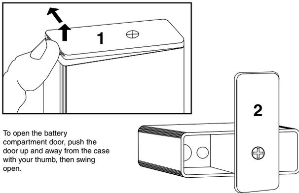
To open the battery compartment door, push the door up and away from the case with your thumb, then swing open.
