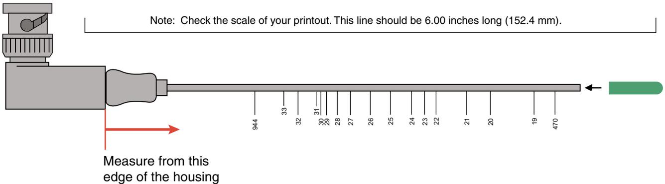
Lectrosonics A500RA UHF transmitter antennas follow the color code specifications in this chart to identify operating frequency block range. (The frequency block range is engraved on the outside housing for each individual transmitter.) If a situation exists whereby the antenna is defective and the antenna cap is missing, refer to this chart to determine the correct replacement antenna.
