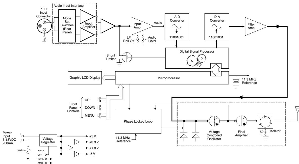
release limiter followed by a slower attack and release limiter. The dual release limiter recovers quickly from brief transients but recovers more slowly from sustained high levels, keeping audio distortion low while preserving short term dynamic changes. When the audio meter on the LCD display widens slightly as it reaches zero, limiting is indicated. When the zero changes to a letter C, severe limiting and/or clipping is indicated.
