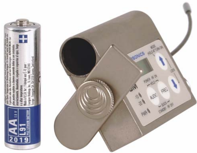
The battery door rotates to open and close. A knurled knob is tightened to hold pressure on the battery contacts.
