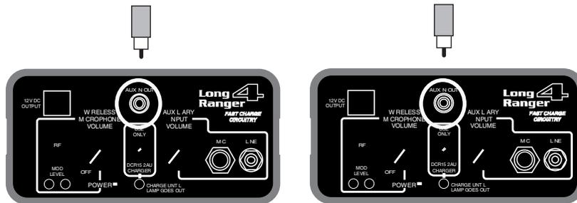
Figure 5 - Connecting Two Long Ranger Systems
