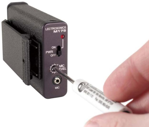
Figure 3 - Transmitter Gain Adjustment
