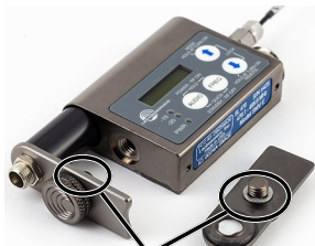
Threads provide electrical contact
