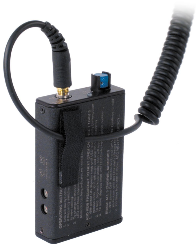
Figure 2 - Headphone cord strain relief
