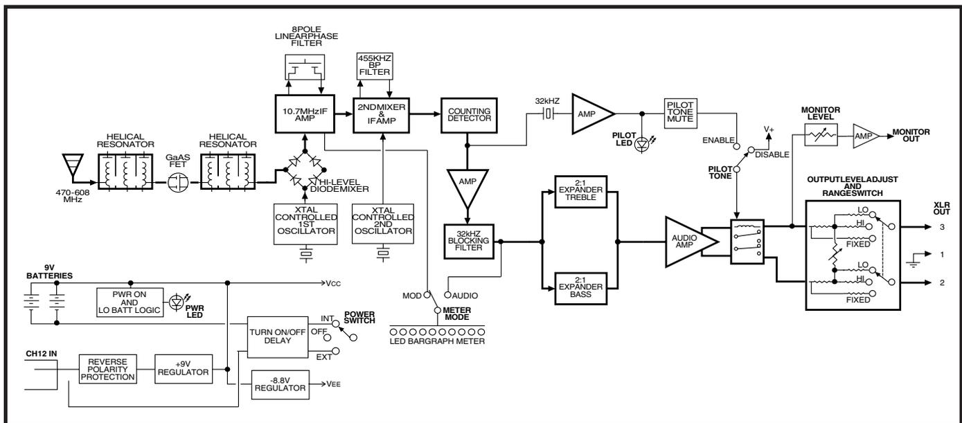
Figure 1 - UCR195 Block Diagram
