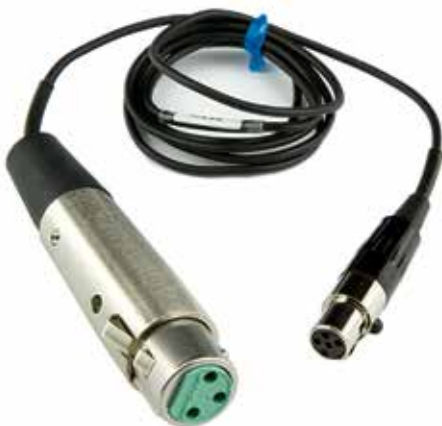
MC35 line level adapter cable. Female XLR to female TA5F; 37 inches long. Feed line level signal to pin 5 on the TA5M jack.
