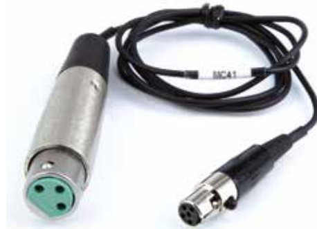
MC41 mic level adapter cable. Female XLR to female TA5F; 37 inches long. Feeds mic level signal to pin 3 on the TA5M jack.
